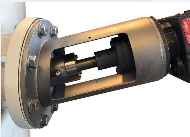
**SHUT OFF DEVICE ENGAGED AND SEAL REMOVED**
