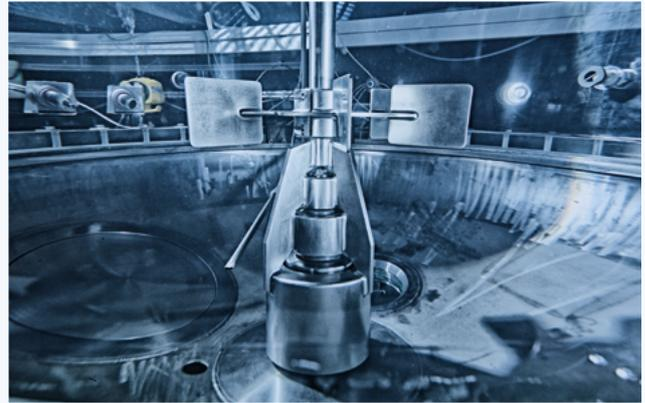
In order to measure the actual power input of each impeller combination into the liquid, it is necessary to know the loss of power generated by the bearing. To do this, the agitator is submersed in water with the water level lying slightly above the agitator shaft. Then the power input of the agitator is measured at different rotational speeds.
