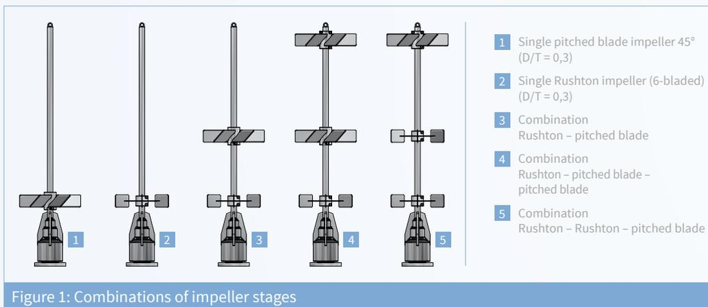
The agitator is driven by a magnetic field, the impeller assembly is located and rides on a bearing shell with ceramic surfaces. In principle, the higher the viscosity and the rotational speed, the higher the power input, whereby also the gassing rate has an influence on this process.
