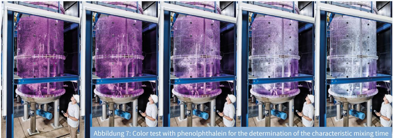
Abbildung 7: Color test with phenolphthalein for the determination of the characteristic mixing time
